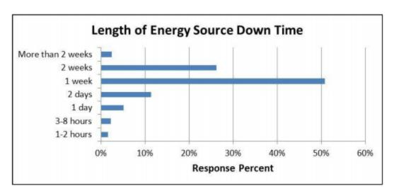
**Figure 4-11: Length of Energy Source Down Time.** This graph is another indicator of the relative vulnerability of the overall energy system in New Jersey. It shows that roughly 80 percent of all energy failures experienced during Superstorm Sandy required at least one week for repair, thus indicating high exposure of energy assets to coastal or at-risk flood areas. Almost 30 percent of the shutdowns required two or more weeks to restore power.
