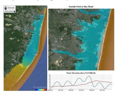
**Figure 4-6: Water Elevation Mapping, Seaside Park to Bay Head, NJ.** Mapping water elevation using the dynamic models developed by Stevens Institute of Technology in partnership with the State facilitates a better understanding of flood risk. These models can be used to asses flood risk under numerous scenarios.
