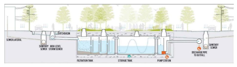
Figure 4-20: Schematic for typical stormwater retention system depicting tanks and typical "High Level" storm sewer system for three DSD sites.
