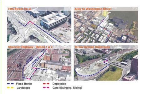
Figure 4-17: Project's Resist alignment features at four locations along alignment.
