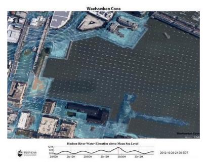
**Figure 4-5: Storm Surge Modeling, Weehawken Cove, NJ.** Modeling the interaction between land and waterways during a storm surge event reveals impacts to public safety, including to evacuation routes and critical infrastructure. These models can be used to understand local risks from storm surges.
